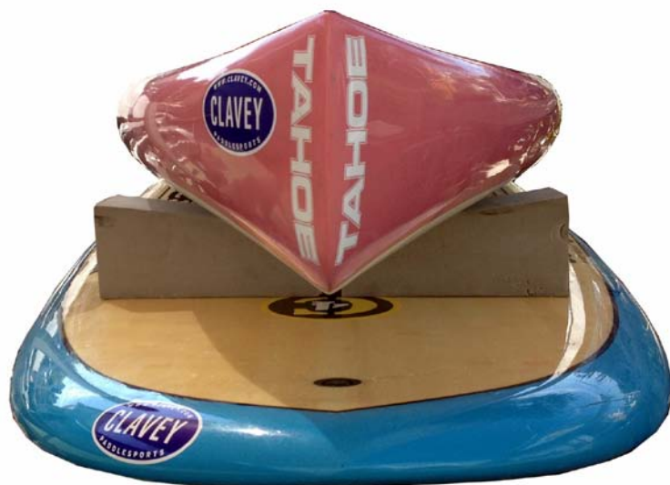
Front view showing the difference between a displacement board (top) and planing board.
